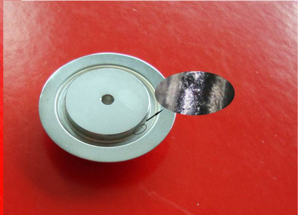
Traditional Shell products (using welding process)
