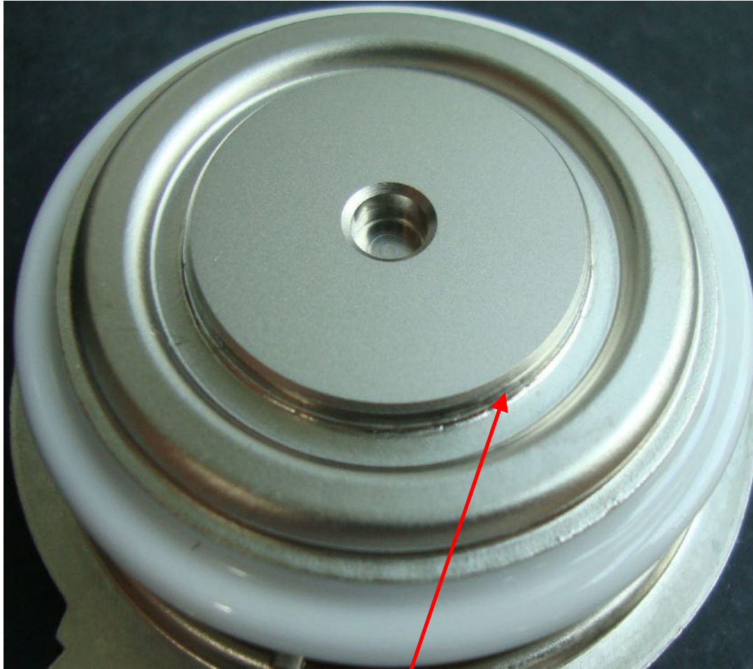
The traditional welded shell anode - welding break point
